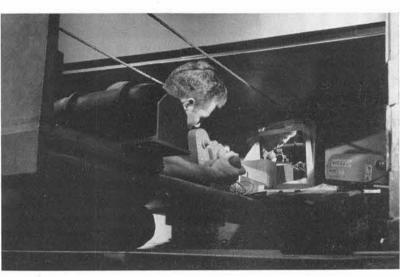
DICK GRAY (8123-3) adjusts Fairchild camera on centrifuge boom before shooting environmental test at Livermore Laboratory. The mirror (rear) is used in filming the opposite side of the test device. The Fairchild camera operates at 64 to 8000 frames a second and the Milliken camera (right) shoots at 400 frames a second.
